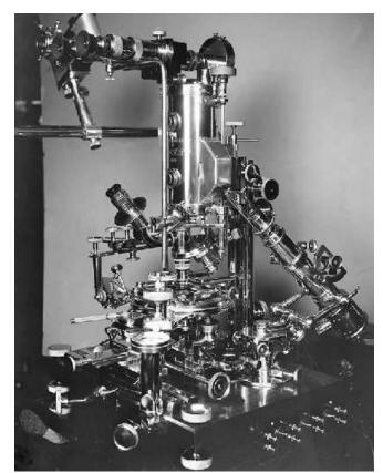
An exact replica of the Universal Rife Microscope (1933), capable of a resolution of 31,000 diameters and a magnification of 60,000 diameters, was able to view the tiny cancer virus (1/15 of a micron in length and 1/20 of a micron in breadth), a feat still impossible with most of today's microscopes.
